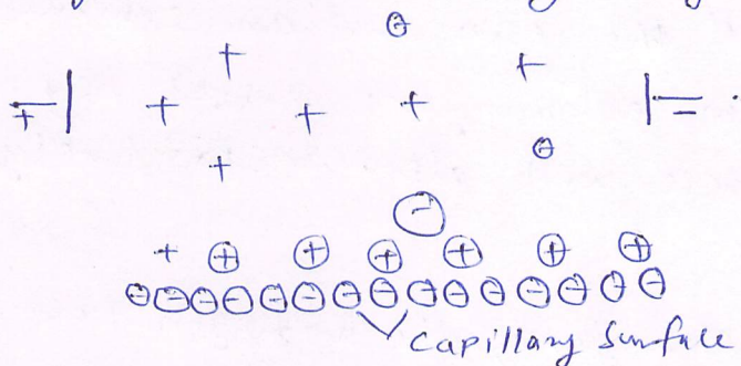
Fig 1 Charge distribution at the silica capillary interface and resulting electroosmotic flow:
